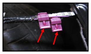
Now plug in the led wires into the back of the quick tap connectors. drivers side: Plug red led wire into purple wire, black to black. Passenger side: Plug red led wire into brown wire, black to black. Don't forget to plug the connectors back into the rear markers before you move on.
