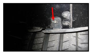
Raise rear of vehicle and support with jack stands. Locate this 7mm screws behind the rear wheels and remove on both sides of car.
