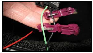
Place one wire in each of the supplied quick tap connectors, fold shut and close with pliers until they latch. The wires you see will be purple or brown and black.
