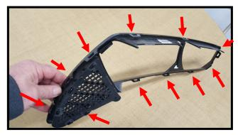
This shows the mounting tabs you are trying to release. There are 3 on top, 4 on the bottom and 2 on each side. Always pull out on the bezel as you are releasing the tabs.
