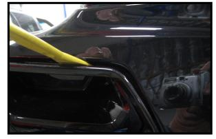
Carefully insert the panel removal tool between the taillight bezel and the rear fascia, pry down while pulling the bezel out. Work your way around the bezel releasing the tabs holding the bezel In place. See next page for clarification.
