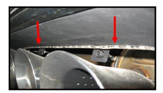
This shows where to mount the exhaust led strip. Clean mounting area with alcohol pad and prep with adhesion promoter before peeling the backing and mounting the strip. Wire tie all the wires up and away from the exhaust. Come back and press the strip into place to be sure it is secure.
