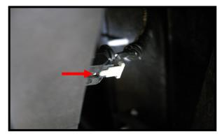
This shows the rear side marker connector. Slide the white tab as shown to unlock the connector from the housing. Pull the connector out so you can wire the leds. If you can't pull the wires out far enough to wire, there are additional harness retainers you can release after removing the tail light bezel.
