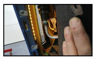
Looking through the quarter panel you can see the lower rear grills. There are 3 tabs on each side you need to release to remove it. Release the bottom ones then pull out while you release the rest of them. Get the top 2 through the tailight opening
