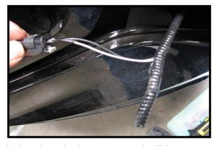
Now split the side marker harness open and pull the wires out for access.
