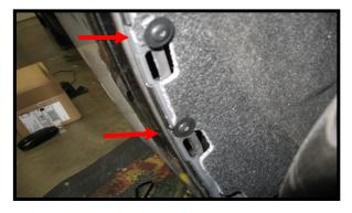
Remove these #15 torx screws behind the splash shield for access to the rear side marker connector. Pull the panel back and secure it with bunge cords to gain access to the rear side marker.
