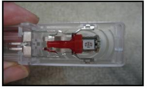
Install the led into the light housing. If it doesn't light, remove it turn it 180 degrees and re-install it. Also make sure the lights haven't timed out which they will do after about 15 minutes.
