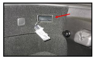
The rear hatch/trunk light housing can be easily removed by prying it out of the panel. Pull out at the red arrow.
