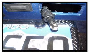
Remove factory bulb. Be careful, it will be hot! Turn on the lights. Insert led bulb. If it doesn't light, turn it 180 degrees and re-install. Reverse this procedure to re-install light and housing. Repeat on the other side.
