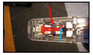
If you are still having trouble getting it to light make sure the factory contact (red arrow) is contacting the small led wire (blue arrow). If they are not contacting each other you can move one or both of them to get contact. After all is working re-install the housings and enjoy the new lights!
