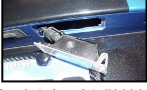
Remove housing from rear fascia. Unlock the housing from the bulb socket by turning it 1/4 turn counter clockwise.
