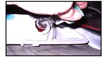
Unlock the reverse light connector by turning it 1/4 turn upward or counter clockwise. Take note of the position of the socket when it comes out . You will need to line up the tabs on the socket with the slots in the housing and turn it 1/4 turn down or clockwise.
