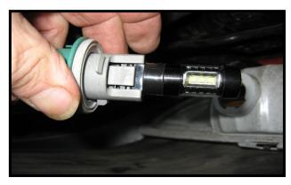
Since the factory wires aren't long enough to pull the socket completely out where its easy to change bulbs, you have to reach up there with both hands to change it. Be patient, it can be done. Have someone start the car and put it in reverse to test. If it doesn't lite up, remove and turn it 180 degrees and plug it back in. Do both leds so you can be sure the brightness is the same on both sides. If one is dimmer than the other remove it, turn it 180 degrees and re install.
