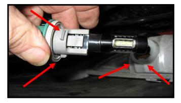
Line up the tabs on the socket with the notches on the housing and once it is all the way in and seated, turn the socket clockwise to lock it in place. Repeat on other side and your done.
