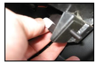
Open the glove box and remove stock bulb from housing. Bulb may be hot. Install LED into housing. If it doesn't lite, turn it 180 degrees and re-install. Bulb should not lite.
