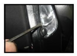
Begin by carefully prying out the map light lens with a small flat screwdriver. Best place to start is near the button.
