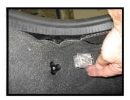
Remove the rear compartment lamps from the carpet.
