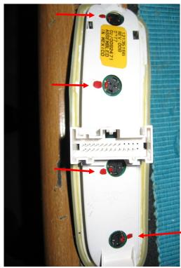
A pair of hemostats with toothed jaws works well for removing the sockets if you need to turn them.
