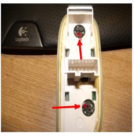
This shows the passenger side leds after they have been turned 1/8 turn into position. Top led in the 6 oclock position and the bottom one in the 9 o clock position. Plug the switch in and test the leds. Hook the bottom of the switch into the door panel and snap switch back into place.
