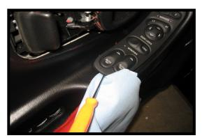
Remove drivers side window switch panel by prying up on the **BOTTOM** of the panel as shown. Remove the passenger side by prying up on the **TOP** OF THE PANEL. You will see 4 small sockets on the drivers side and 2 on the passenger side. Simply turn them 1/8 turn counter clockwise and remove all 6 factory bulbs. Refer to the diagram below for installing the LEDs.
