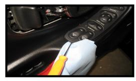
Remove drivers side window switch panel by prying up on the **BOTTOM** of the panel as shown. Remove the passenger side by prying up on the **TOP** OF THE PANEL. You will see 4 small sockets on the drivers side and 2 on the passenger side. Simply turn them 1/8 turn counter clockwise and remove all 6 factory bulbs. Refer to the diagram below for installing the LEDs.
