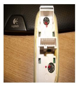
This shows the passenger side leds after they have been turned 1/8 turn into position. Top led in the 6 oclock position and the bottom one in the 9 o clock position. Plug the switch in and test the leds. Hook the bottom of the switch into the door panel and snap switch back into place.
