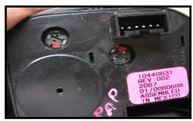
Red arrows show the location of the 2 bulbs. Using a good fitting flat screwdriver, turn the bulb counterclockwise 1/8 turn and remove.
