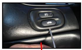
Locate the slot in the bottom of the hatch/fog housing.
