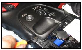
Open the center console. Using a small pry tool pry the A/H Panel up and out of the console. Disconnect the wiring harness.
