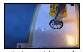
Using your thumb, press the leds into place firmly. Using a flat bladed screwdriver that fits the slot well, twist clockwise 1/8 of a turn until it locks into place. Using the same procedure as on the hatch switch, install the leds and twist them into place. Turn on the lights and plug the panel in to test. If they don't light remove the led, turn it 180 degrees re-install.
