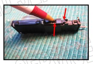
Release the connector from the housing by depressing this tab at either arrow then disconnect the light. You can put the light back in the housing but it wont be used.
