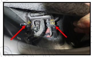
Re-install the light housing by lining up the clips with the bracket openings. Support the bracket from behind while pushing the light housing back In place.
